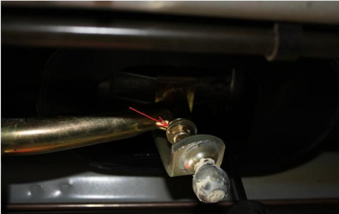
Remove the four 4mm Allen head bolts (see red paint in photo below). In this photo, you may notice that the shift rod is still on the fork. You can remove the e-clip as described above after the 4 Allen bolts are removed... either way is OK.
