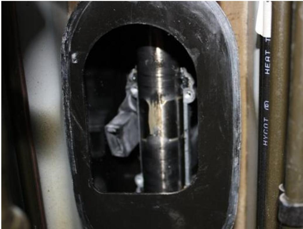
Remove the e-clip from the shift fork. This is exactly the same as the clips/washers you removed earlier. Photo below shows these clips removed. Slide the fork and shuttle half off of the shift lever.
