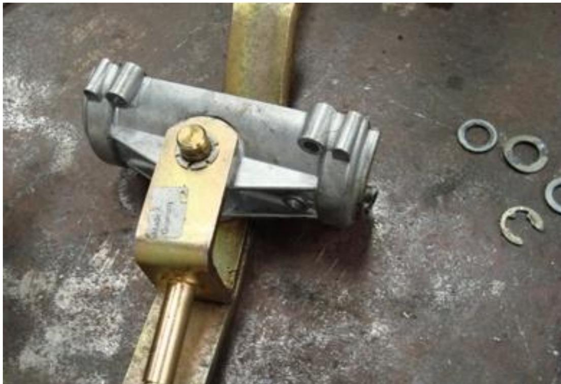
Slide the fork off of the shuttle half *being careful to retain the rubber o-rings*.
