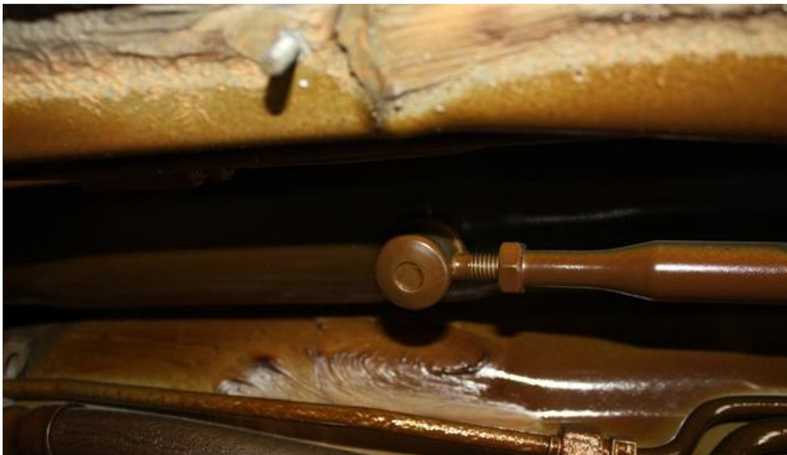
Use a small screw driver to pry off the e-clip. There will be 3 washers (2 flat and one wavy). The wavy washer is sandwiched between the 2 flat washers and keeps tension on the e-clip and bushings. Slide the shift rod and rubber boot out of the way.
