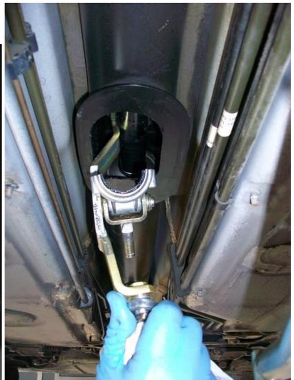
When the shift lever and shuttle half are almost in place, slip the upper shuttle half in the opposite side of the opening. The goal is to just get it up there at this point.
