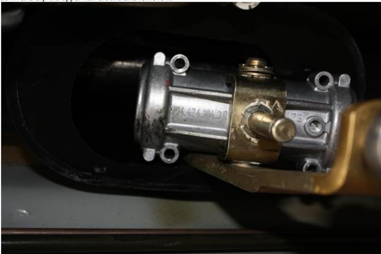
Slide the shift lever down and carefully pull from the upper rubber boot. Take this assembly to a workbench.
