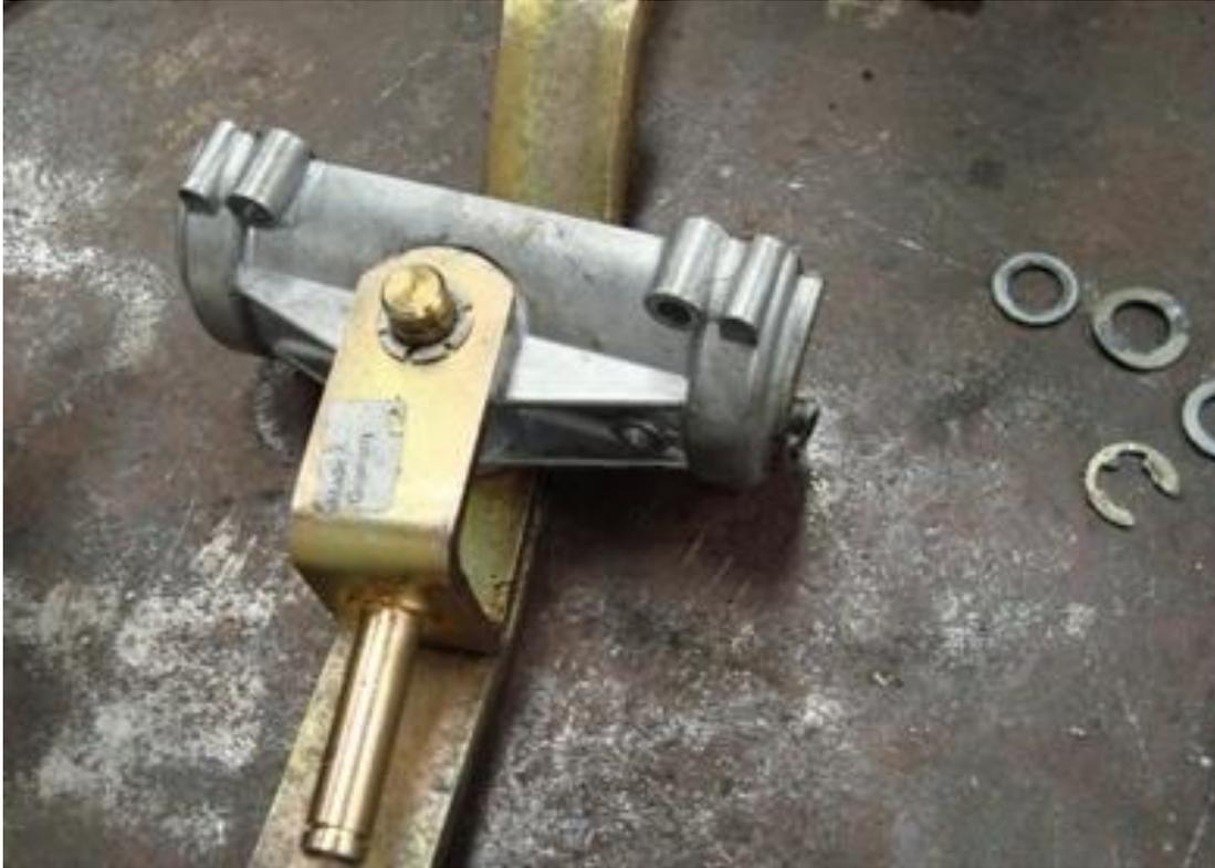
Slide fork off of the shuttle half being careful to retain the rubber o-rings.
