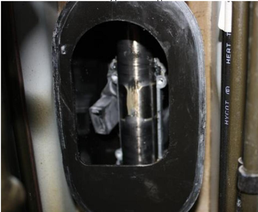
Remove the e-clip from the shift fork. This is exactly the same as the clips/washers you removed earlier. Photo show these clips removed.
