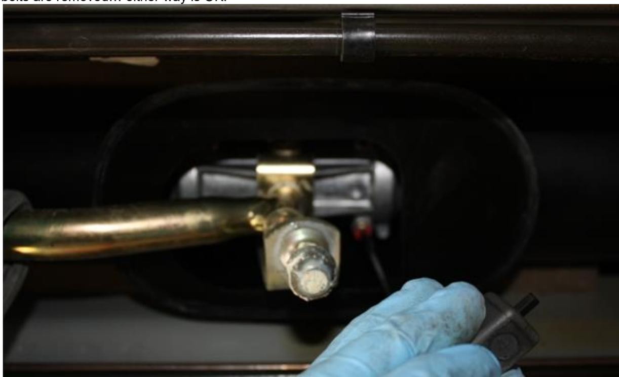
Separate the shuttle halves (This probably already happened). Let the lower half that is attached to the shift lever/fork drop down and slip the upper half around and remove it.
