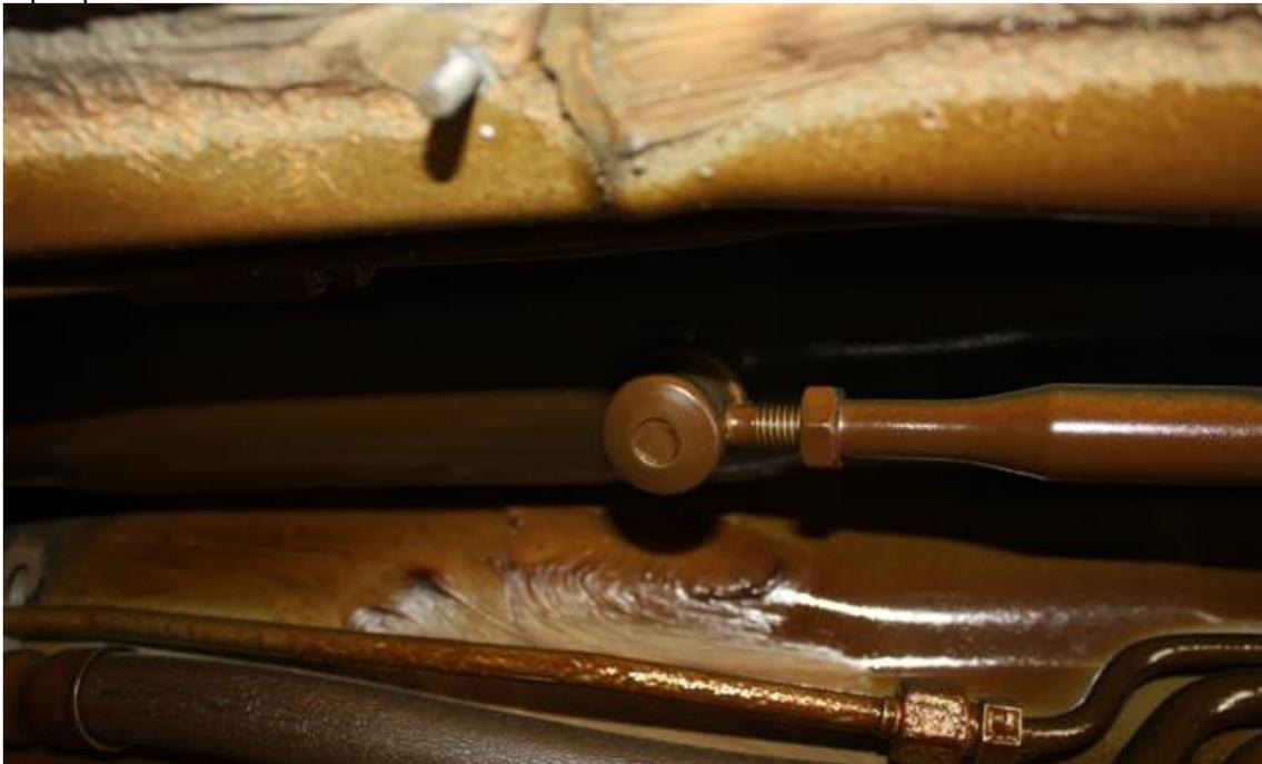
Use a small screw driver to pry e-clip off. There will be 3 washers (2 flat and one wavy washer). The wavy washer is sandwiched between the 2 flat washers and keeps tension on the e-clip and bushings. Slide shift rod and rubber boot out of the way.
