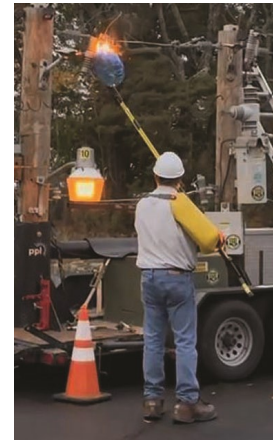
Larry Cheslock demonstrating the effects of a mylar balloon with live wire contact.
