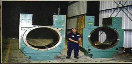
*Bearing chuck completely rebuilt*
