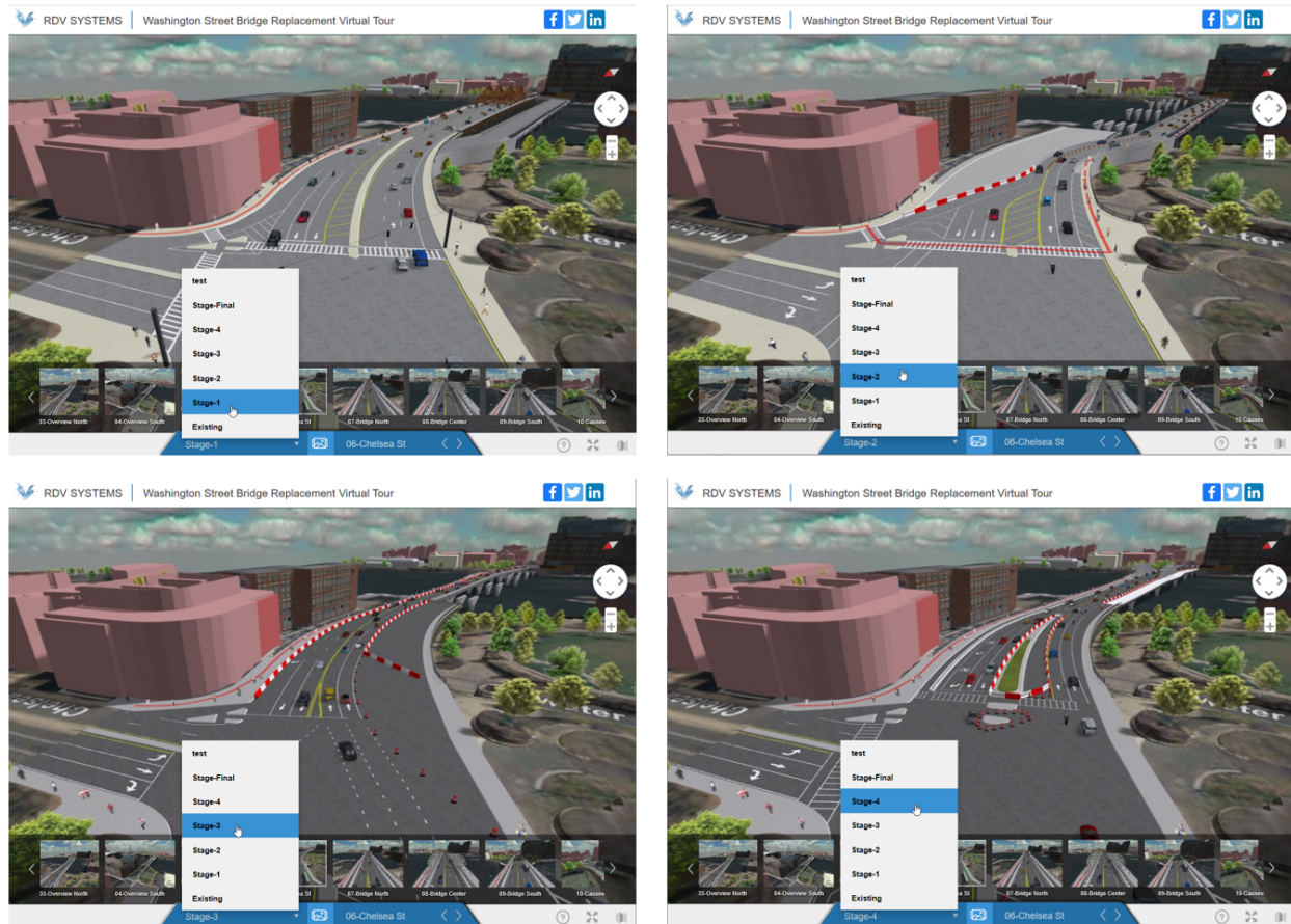
Figure 4 – Virtual Tour Showing Maintenance-of-Traffic Details for Multiple Construction Stages
