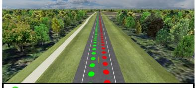
Existing No Pass; Analysis Indicates Passing OK Existing Passing; Analysis Indicates No Passing
