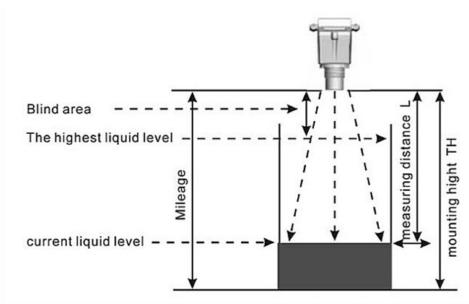
As shown, instrument's transducers made after the wave hit the level reflected back to transducer, the transducer receives income calculated after the hair waves to waves of time, are measured from the L, meter installation height minus the measurement of TH the distance L will be the current level H.
