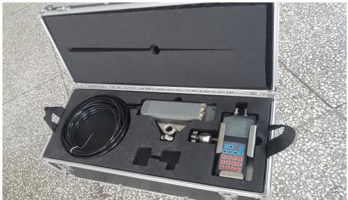
The product measures the flow rate according to the principle of ultrasonic Doppler effect, and can measure the water level through the pressure sensor and the temperature sensor to measure the water temperature. The shell is made of PVC plastic, which can effectively waterproof and seal. The internal power supply is 12V rechargeable battery.
