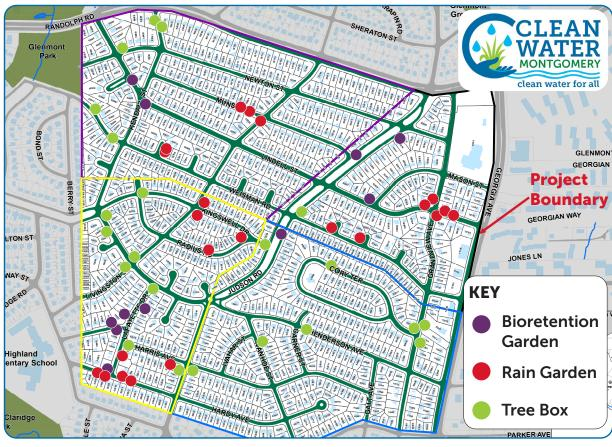
The Glenmont Forest Green Streets project includes multiple small-scale projects including tree boxes, bioretention gardens and rain gardens installed in the County rights-of-way to capture water from roadways, driveways, and sidewalks during storms.
