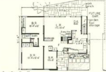
1951—York's second prizewinner in the Long Island Home Builders Institute contest drew an average of five times as many inquiries as the more modern first place design. Innovations: split bath, two-way fireplace, rear living room.
