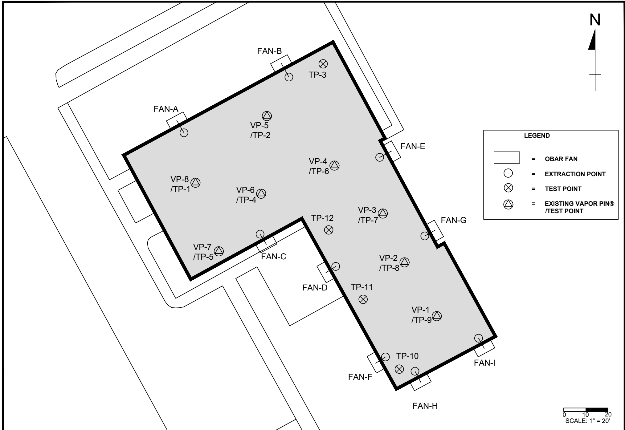
PROPERTY MAP WITH SUB-SLAB DEPRESSURIZATION SYSTEM AND TEST POINTS
