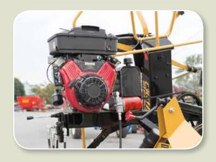
Powerful 16 HP 2 cylinder Vanguard engine easily handles heavy crops such as rye, oats, triticale, etc. Also works great on corn fodder, straw, etc.
