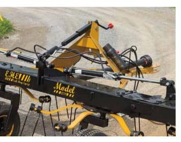
Hydraulic tilt allows operator to lift tedder over rocks, ridges, etc. while in operation.
