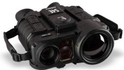
The PR110 MF is a sophisticated, yet user-friendly, and portable handheld thermal imager that is perfect for ground applications due to its ease of use and maintenance. It has the ability to see through fog, smoke, and darkness, making it a valuable tool for a wide range of activities.
