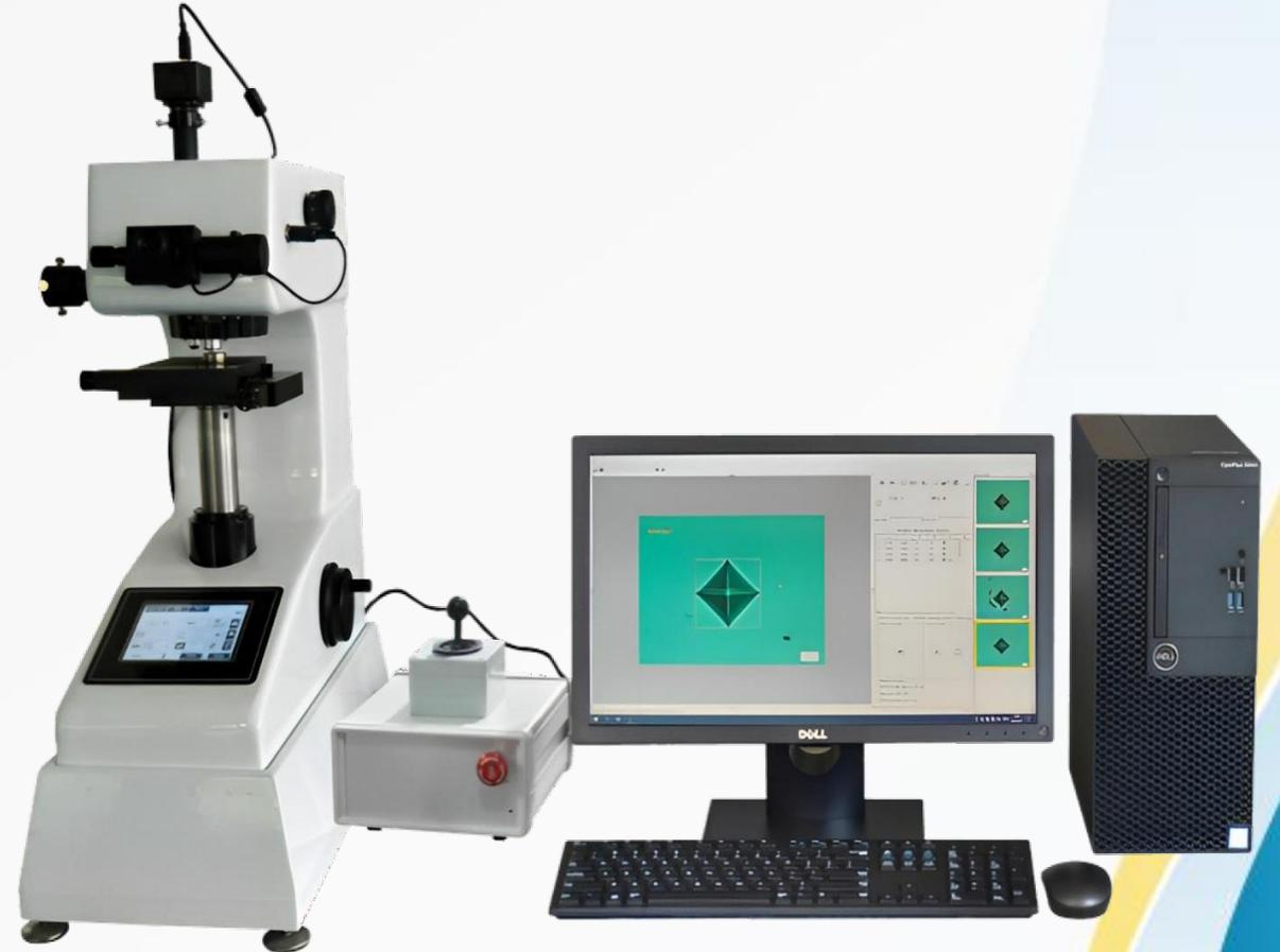
5. Hardness curve, Statistics, Auto-alarm: Automatically detects and plots multiple hardness curves and calculates the hardness case depths. Automatically updates the statistics such as average, min and max, standard deviation, Cp, and Cpk; Automatically marks data that are out of specification limits; May load the depth template file for convenience.
