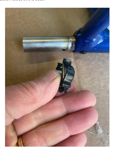
Slide the foot section onto the connection tubes of the main chassis until the holes align and insert the frame clips fully:
