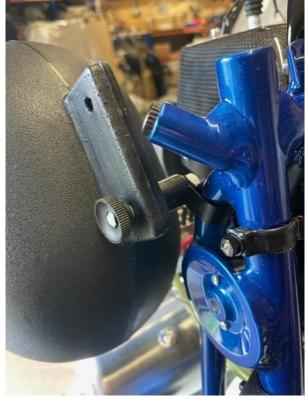
Step 9: Fit the harness top mount attachment screws through the holes in the top of the frame, don't overtighten the bolts or you will crack the plastic clamps!
