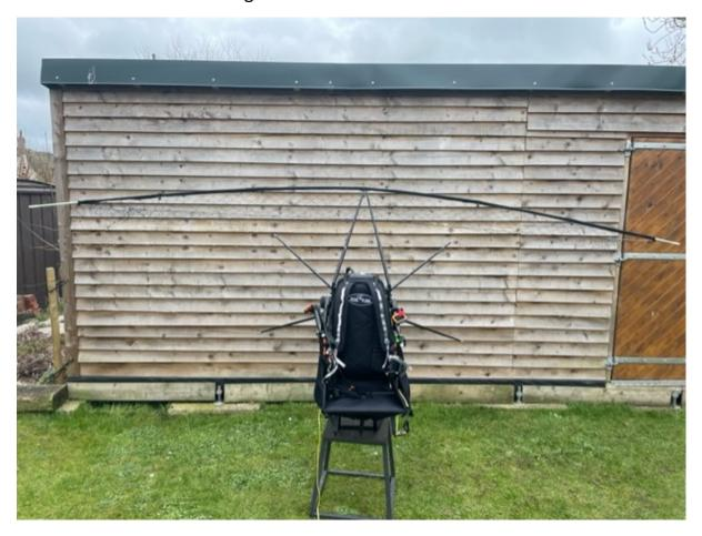
Again, working one side at a time, Brace the main frame with one hand, grasp the end of the fibre pole with your other and bend it round to slide into the hole in the base section. You may need to use your elbow to push down on the pole to form the ring. Have a look at the <u>video</u> to help you
