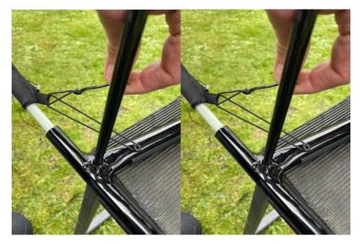
Then tension the inner chord, on the end of each side of the inner chord you will find a small carabiner/maillon and approx. 30cm along the chord a steel ring. Standing on the engine side of the frame, take the ring on the right side of the chord, pass it under the fuel tank and place it over the hook on the left hand upright:
