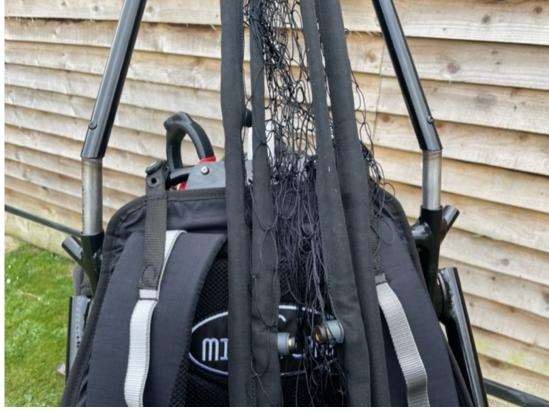
Use the frame clips to secure the upper sections in place.
