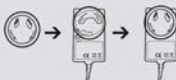
Step 3: Install the corresponding adapter head for your regions and connect to the power supply
