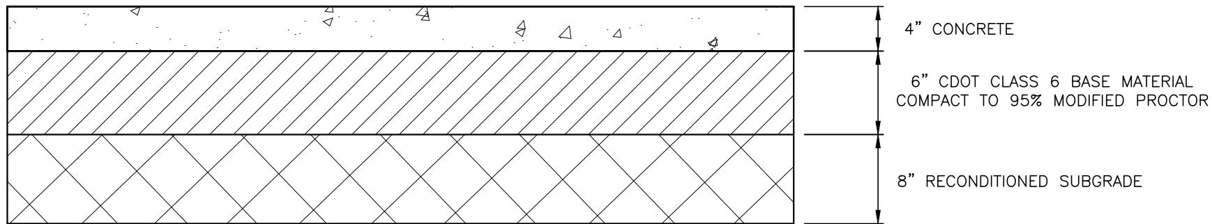
TYPICAL SIDEWALK CONCRETE THICKNESS DETAIL N.T.S.
