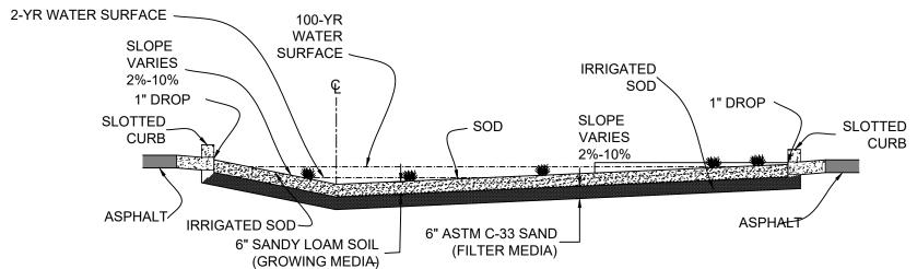
1. IRRIGATION HEADS WILL NOT BE PLACED BELOW THE 2-YEAR SURFACE ELEVATION. 2. SEE CALCULATIONS TO SHOW CAPACITY. ENTIRE SYSTEM IS PART OF WATER QUALITY SYSTEM.
