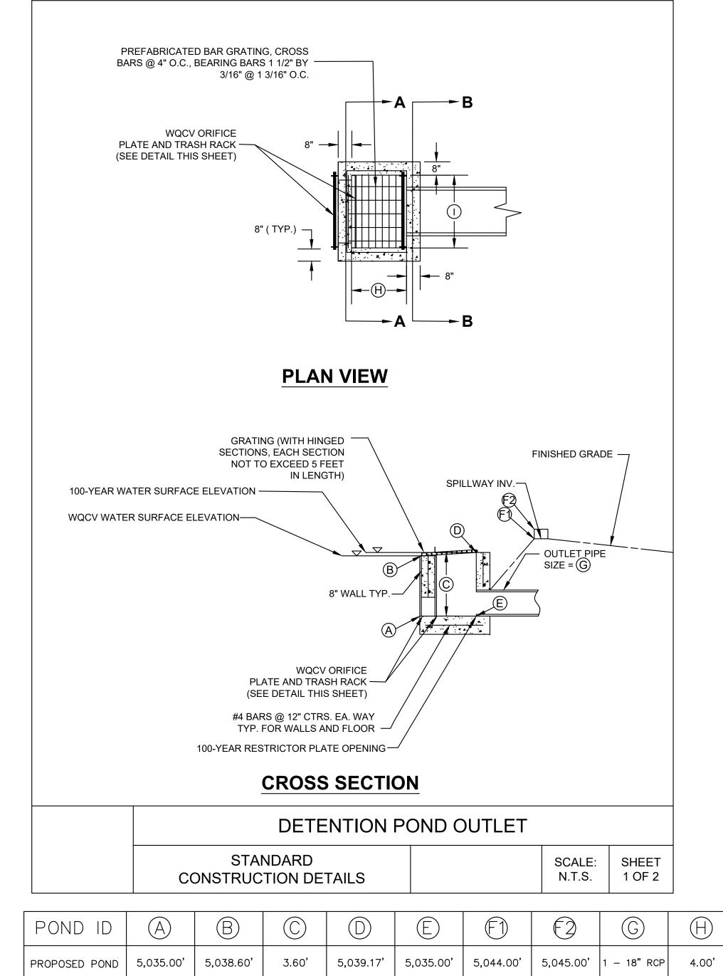
NOTE: THIS TABLE REFERS TO THE ABOVE "DETENTION POND OUTLET" CONSTRUCTION DETAIL
