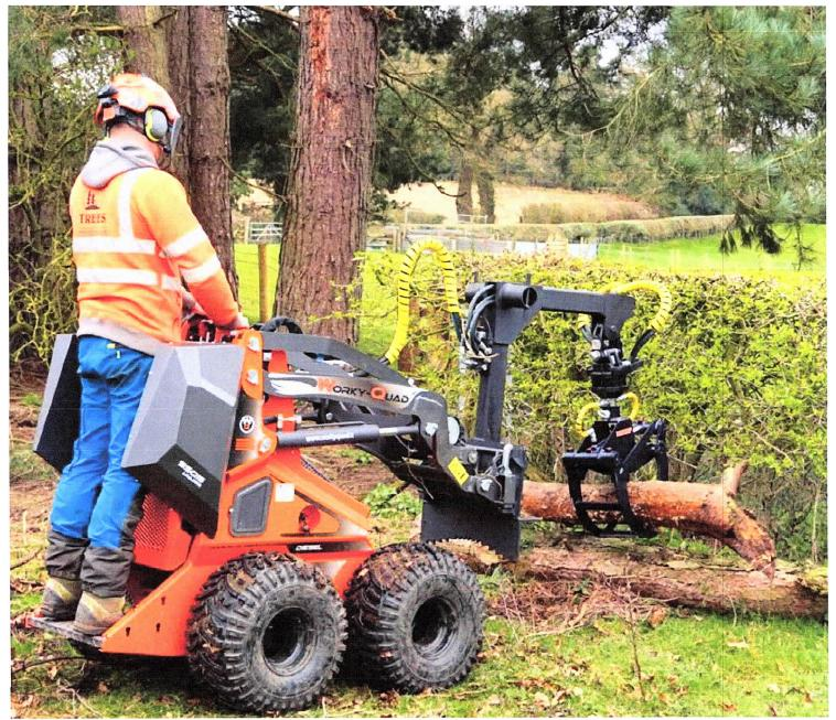
Keep the load low and slow for greater stability, as low as possible and as slow as necessary with respect to the terrain. Shown here is a Worky-Quad SSQ15 loader. Photo courtesy of Branch Manager Attachments. »
