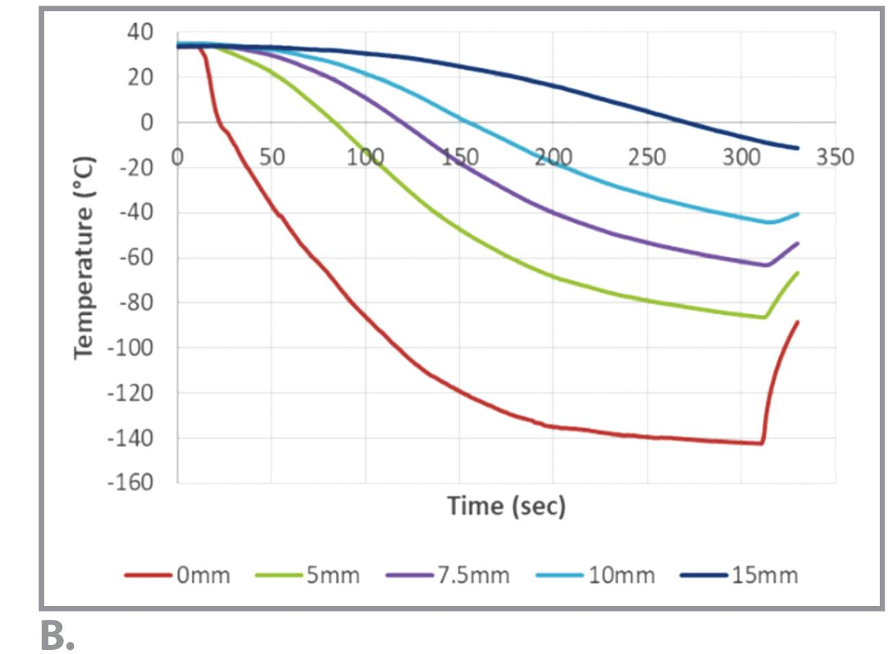
**Figure 3**. Real-time monitoring of the isotherm profiles generated by the (A) cylindrical and (B) coiled cryoprobe prototype at the center of the ablation segment during a 5.5-min freezing cycle.
