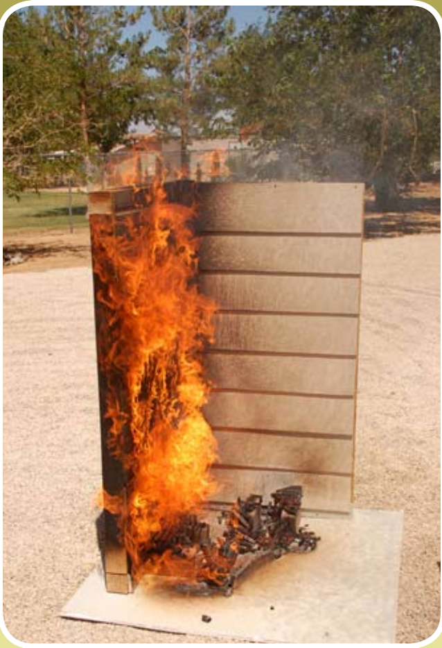
Vertical flame spread on a combustible siding product. The right-hand side of the wall is constructed of noncombustible siding. Both wall sections had the same initial fire exposure.
