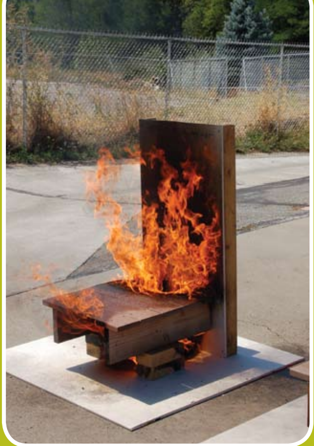
The decking being tested here doesn't comply to Chapter 7A provisions.
