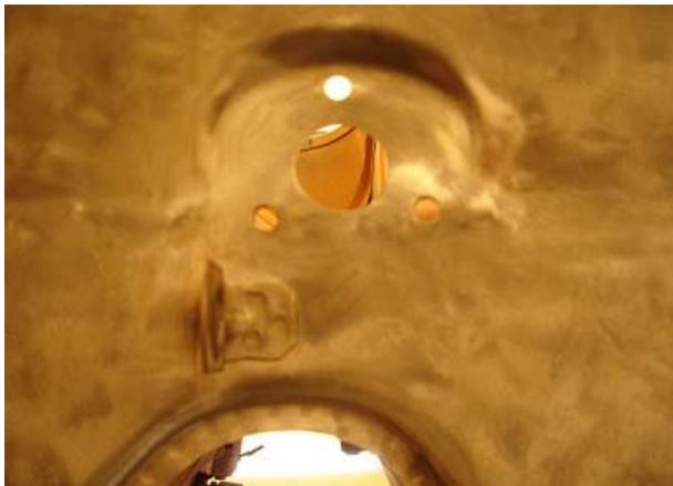
Step 2. Before attaching the panels, check the chassis and repair all rust or cracks, especially around all production welds and where two or more panels come together. Below you see how the chassis has been stressed by the sway bar and has cracked by the top bolt hole. This crack and the holes should be welded and ground down as new holes will need to be drilled for the new stiffening panels.
