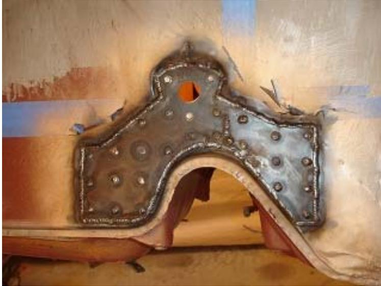
Step 7. You're now ready to re-weld the brake line bracket back on. Once you are done welding and depending on how good of a welder you are, you will need to grind all those welds flat!
