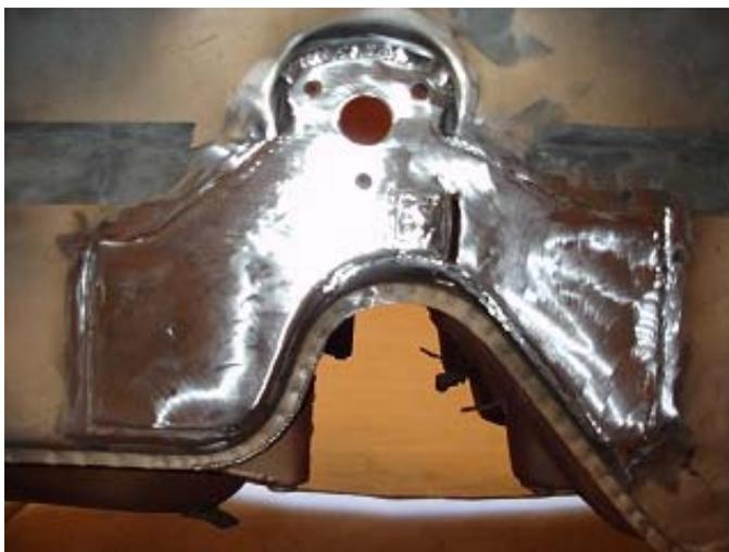
Step 8. When you're done grinding down your welds, drill out the holes for the mounting bolts and sway bar. Finally, give it a nice coat of primer and paint, depending on where you live you may also want to apply some undercoating. Have fun and good luck!
