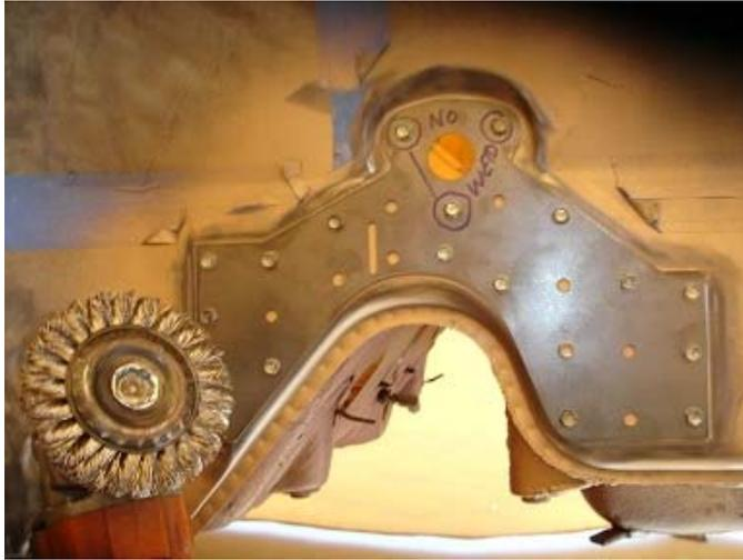
Step 6. Now start at one end of the panel, remove one screw at a time and fill each hole with a weld. After each weld blow some air on the weld to cool it then move to another part of the panel and repeat; this will help spread the heat out as to not put too much stress on the chassis.
