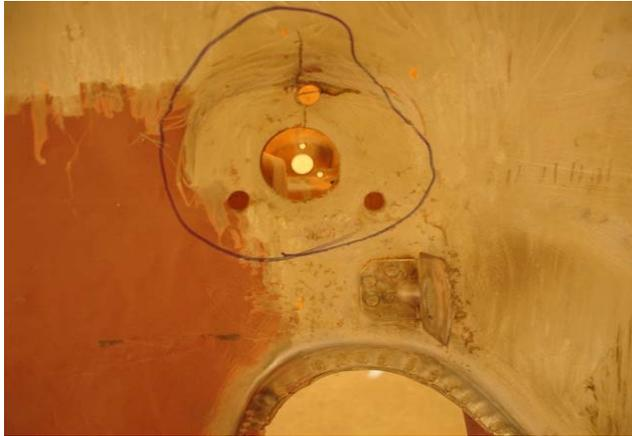
At this point you need to decide whether or not to remove the brake line bracket and then re-weld it on top of the stiffener panel or use the slot provided so the panel can slip over the bracket. In this installation the bracket was removed and re-welded for a nice flush look. You can get a special tool that cuts around the spot welds or you can simply drill them out and use a cold chisel. Be sure to take some measurements and a couple of pics before you remove.
