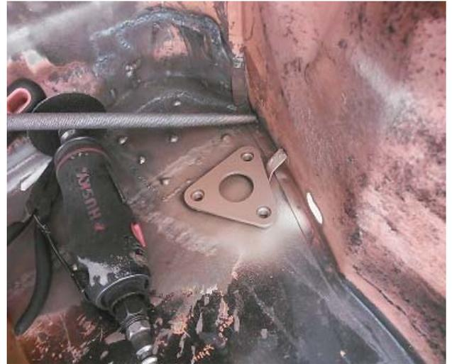
Step 1. Areas to be welded must be cleaned of all undercoating, dirt and grease. Some tools you will need are a small cut off wheel, rat tail file, 3/8" drill bit and probably some pliers.
