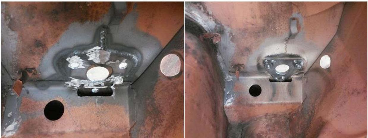
Step 8. Now weld around the edges as shown. After each weld blow some air on the weld to cool it then move to another part of the panel and repeat, this will help spread the heat out and not stress the chassis.
