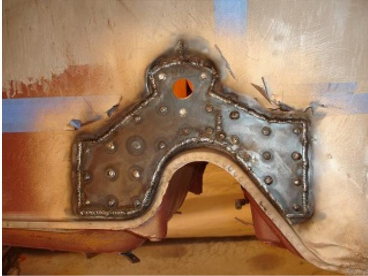
Step 7. Re-weld the brake line bracket back on now. Once you are done welding and depending on how good of a welder you are, you will have to grind all those welds flat!
