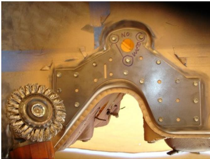
Step 6. Now start at one end of the panel and remove one screw at a time and fill the hole with weld, after each weld blow some air on the weld to cool it then move to another part of the panel and repeat, this will help spread the heat out and not stress the chassis.
