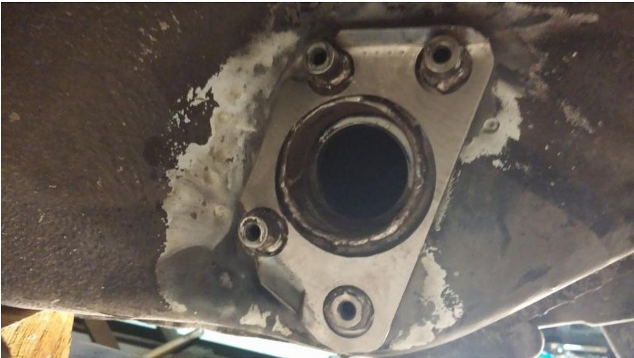
Step 5. Once you are satisfied with the placement, and to ensure that the stiffening panel is held tight to the body, you will want to drive a couple of #10 self-tapping sheet metal screw in and use clamps where ever possible. I know it is a lot of work but the reason for driving a screw in is to hold the panel in place while you weld and when you remove the screw it leaves a nice little hole to weld the two panels together.
