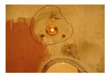
Step 3. At this point you have to make a decision if you want to remove the brake line bracket and then re-weld it on top of the stiffener panel or use the slot provided so the panel can slip over the bracket. In this installation the bracket was removed and re-welded for a nice flush look. You can get a special tool that cuts around the spot welds or you can simply drill them out and use a cold chisel. Make sure to take some measurements and a couple of pics before you remove.
