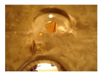
Step 2. Before attaching the panels, check the chassis for cracks, especially around all productions welds and where two or more panels come together, and repair any cracks or rust. Below you see how the chassis has been stressed by the sway bar and has cracked by the top bolt hole. This crack and the holes should be welded and ground down as new holes will be drilled for the new stiffening panels.
