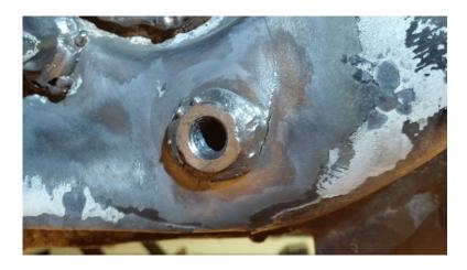
Step 3. Once any repairs are made and all undercoating has been removed, you need to prep the bare metal with a weld-able primer. A good product is SEM Copperweld 40783.
