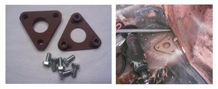
Step 1. Areas to be welded must be cleaned of all undercoating, dirt and grease. Some tools you will need are a small cut off wheel, rat tail file, 3/8" drill bit and probably some pliers.
