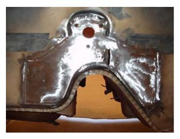
Step 8. When you're done grinding down your welds, drill out the holes for the mounting bolts and sway bar. Finally, give it a nice coat of primer and paint, depending on where you live you may also want to apply some undercoating. Have fun and good luck!
