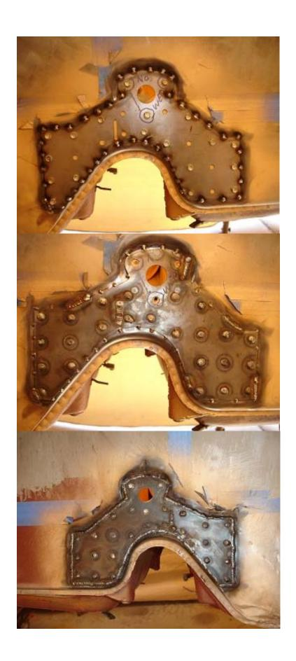
Step 7. You're now ready to re-weld the brake line bracket back on. Once you are done welding and depending on how good of a welder you are, you will need to grind all those welds flat!
