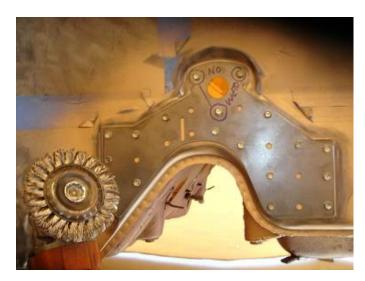
Step 6. Now start at one end of the panel, remove one screw at a time and fill each hole with a weld. After each weld blow some air on the weld to cool it then move to another part of the panel and repeat; this will help spread the heat out as to not put too much stress on the chassis.
