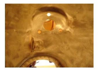
Step 2. Before attaching the panels, check the chassis and repair all rust or cracks, especially around all production welds and where two or more panels come together. Below you see how the chassis has been stressed by the sway bar and has cracked by the top bolt hole. This crack and the holes should be welded and ground down as new holes will need to be drilled for the new stiffening panels.
