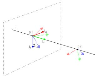
Here you can see the axis directed from the first point towards the second point, constitutes the y-axis of the line coordinate system. The z-axis is defined by the projection of the z-axis of  $p1$  onto the plane perpendicular to the line. The position of the line coordinate system is the same as the position of  $p1$ .
