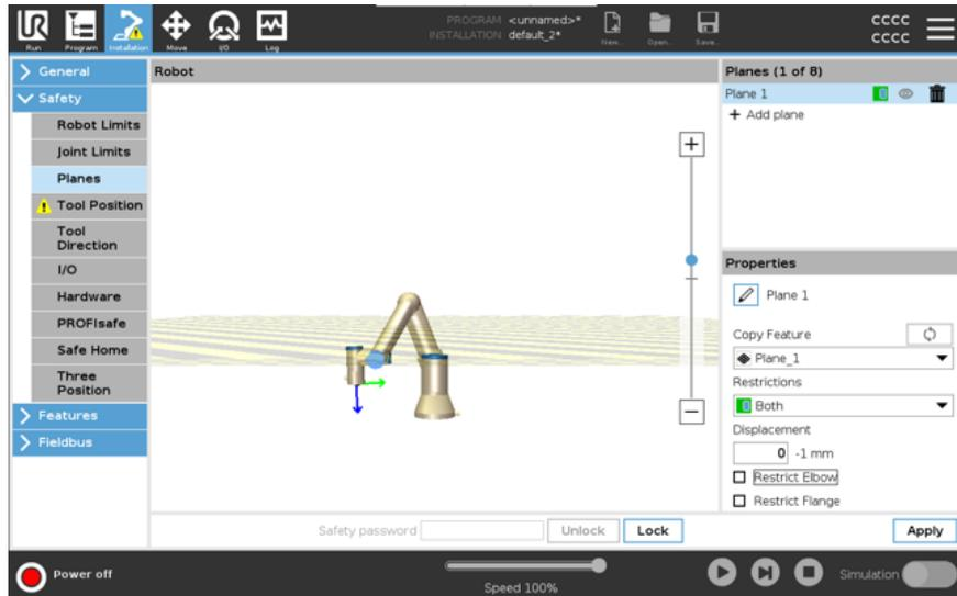
The unrestricted tool flange can cross a safety plane, even when no tool is defined. If no tool is added, a warning on the Tool Position button prompts you to correctly define the tool. When working with an unrestricted tool flange and a defined tool, it is ensured that the dangerous part of the tool can't go above and/or beyond certain area. The unrestricted tool flange can be used for any application where safety planes are needed, like Welding or Assembly.
