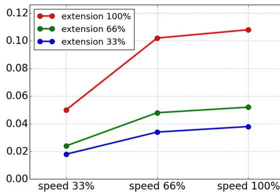
Stopping time in seconds for 66% of 16kg
