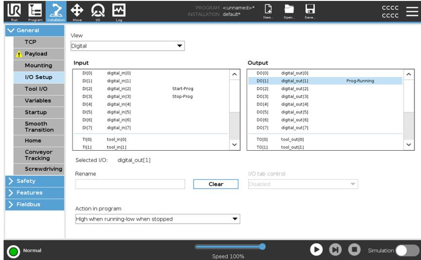
**I/O Signal Type** To limit the number of signals listed under **Input** and **Output**, use the **View** drop-down menu to change the displayed content based on signal type.
