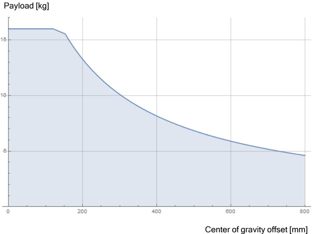
**2.3:** *The relationship between the rated payload and the center of gravity offset.*
