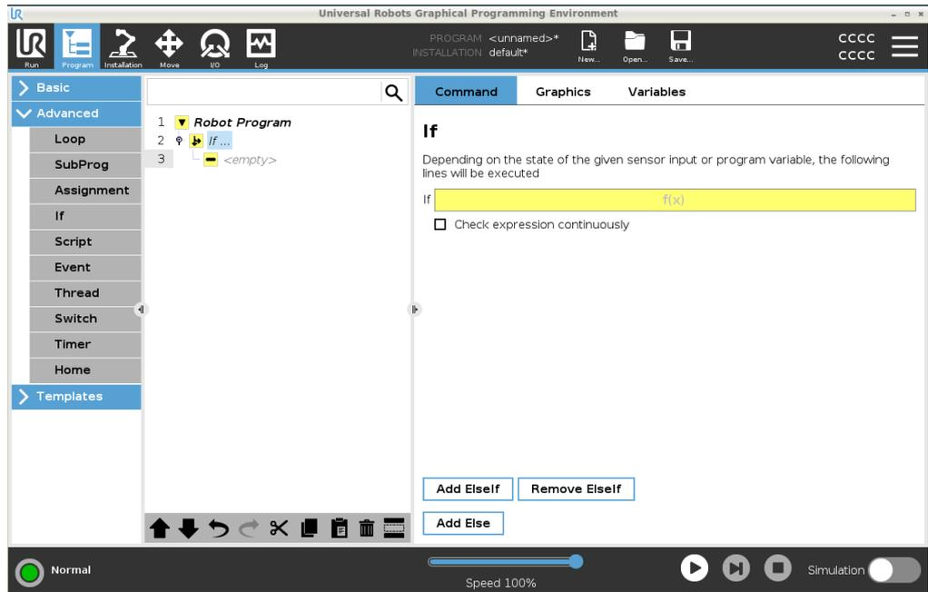
**Example** You can use the If command to create two different results for a robot program.
