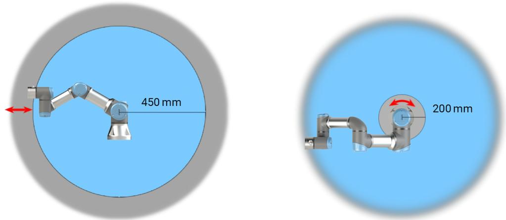
**2.1:** *Due to the physical properties of the robot arm, certain workspace areas require attention regarding pinching hazards. One area (left) is defined for radial motions when the wrist 1 joint is at least 450 mm from the base of the robot. The other area (right) is within 200 mm of the base of the robot, when moving tangentially.*
