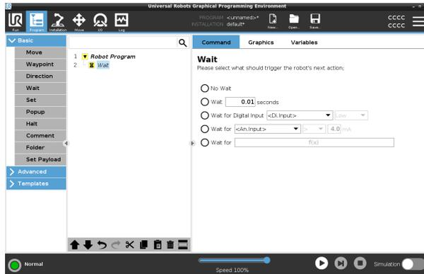
**Example** You can use the Wait command to make the robot program wait for a signal from a sensor that is attached to the control box.
