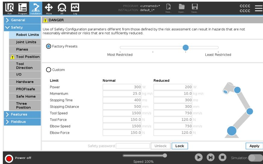
**Custom** Custom is where you can set Limits on how the robot functions and monitor the associated Tolerance.
