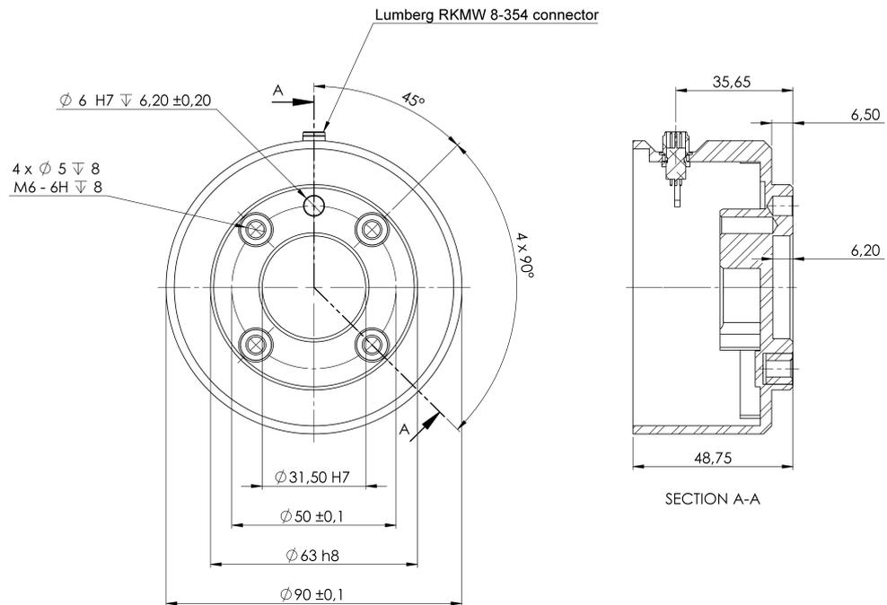
2.2: Dimensions and hole pattern of the tool. All measurements are in millimeters.
