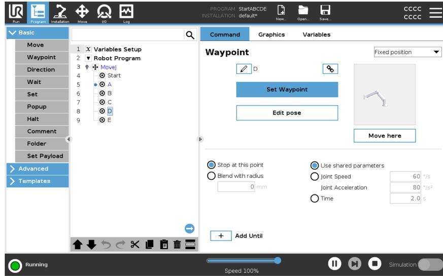
When the program is running, the program node currently being executed is indicated by a small icon next to that node.
