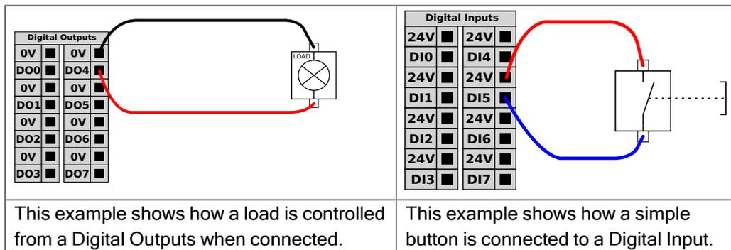
**Communication with other machines or PLCs** You can use the digital I/O to communicate with other equipment if a common GND (0V) is established and if the machine uses PNP technology, see below.
