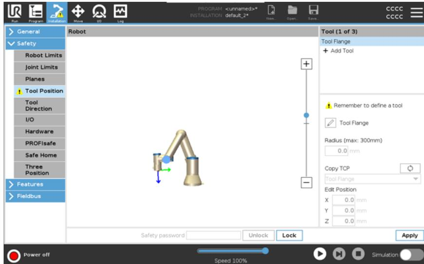
Tool Position button without the warning indicates a tool (other than the Tool Flange) is added.
