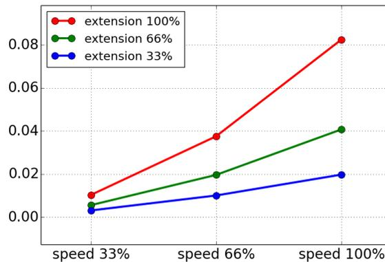
Stopping distance in meters for 66% of 16kg
