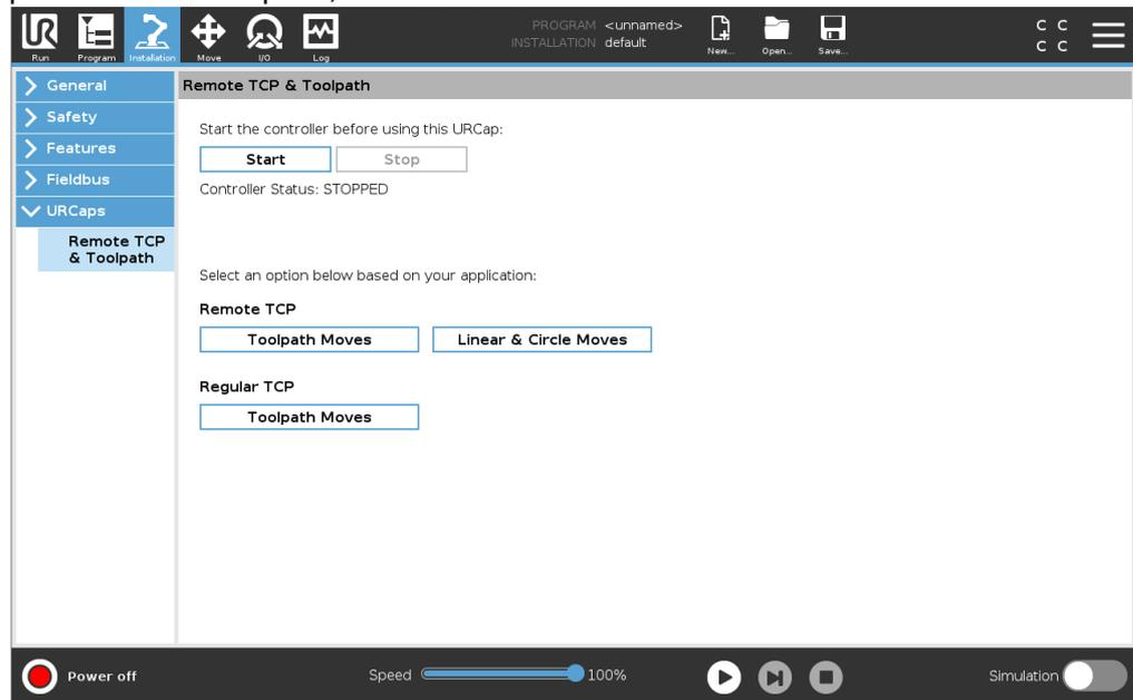
Similar to a regular TCP (see ) you can define and name an RTCP in the Installation Tab's Setup.
