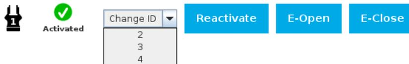
Fig. 4-11: Gripper ID modification in the Gripper Dashboard
