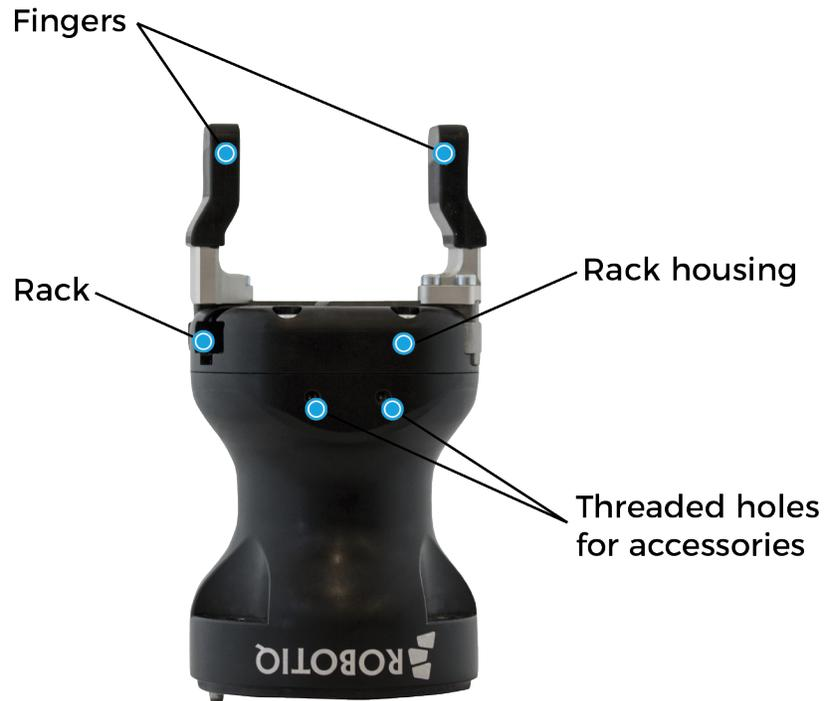
*Fig. 1-1: Robotiq Hand-E Gripper.*
