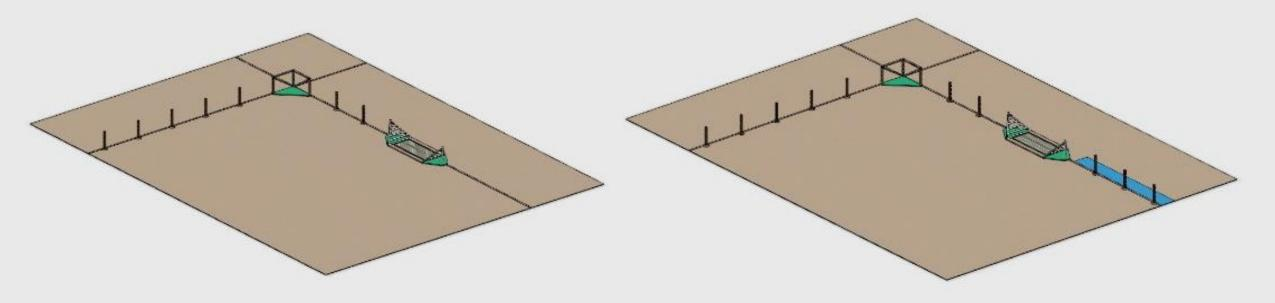
• If desired, install a cattle guard (part # CG-001) or a single wooden gate (part # WG-003). Glue it in place with white glue, centered on the fence line and equal distance as the post settings. Be sure the notches on the posts align with the other posts as you will be installing a strip of straight wire onto them.
