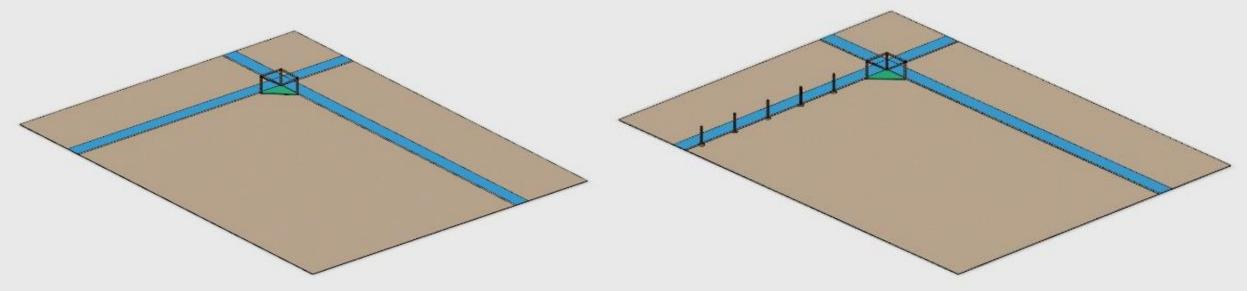
Use a white glue to install the corner post assembly along the inside line. Doesn't need much glue. I use either Elmer's or Woodland Scenics Scenic Glue. I'll use square posts for this diorama. Use a
