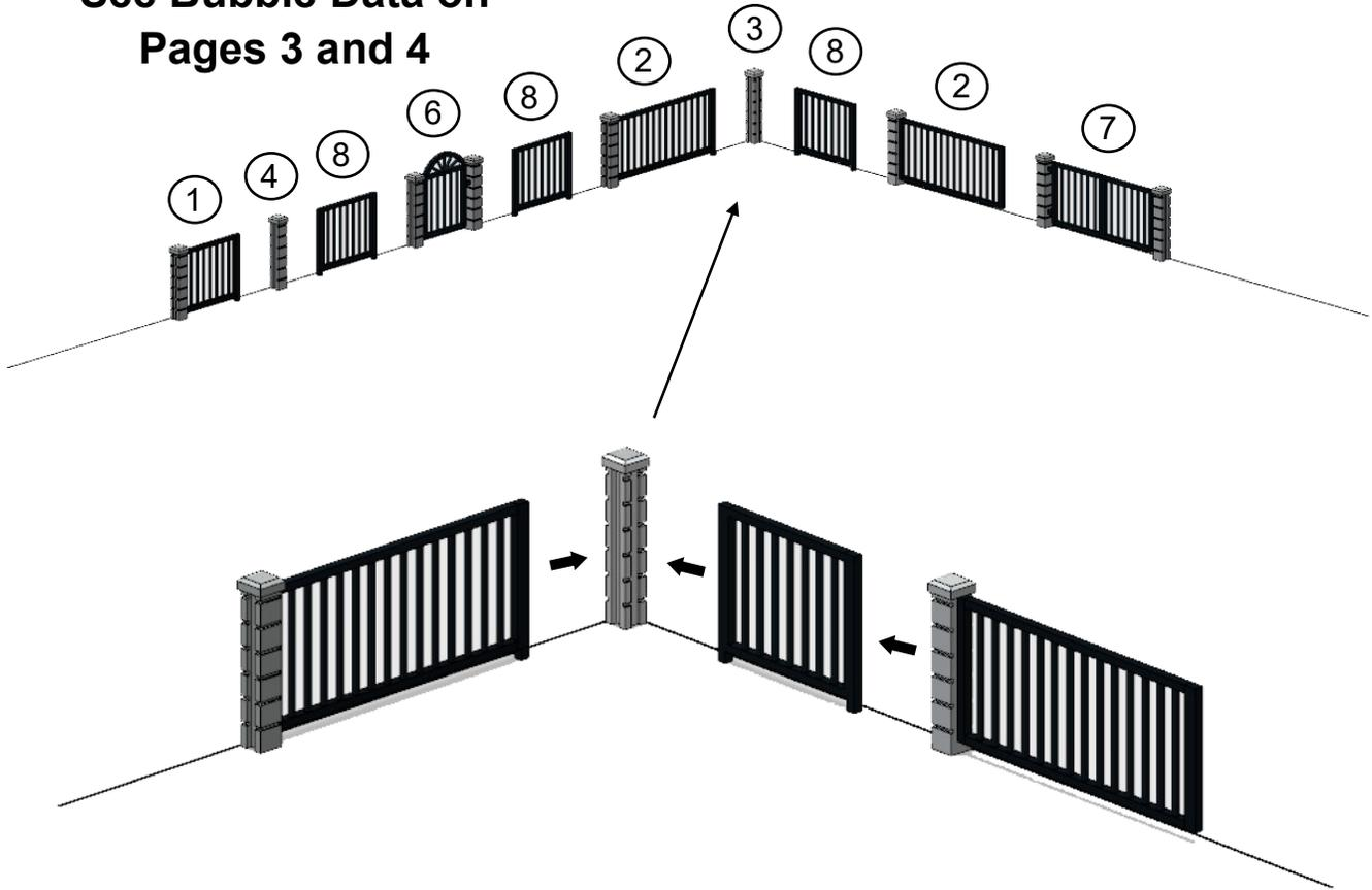
**Draw perpendicular construction lines on your layout at the point where you wish to start installing the fence. The lines will help keep the wall straight during installation.**
