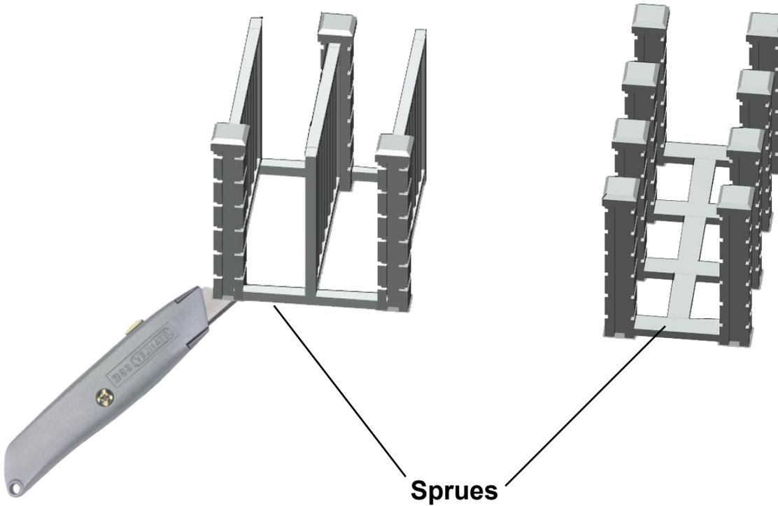
**Cut away all of the connector pieces (sprues) with a utility Knife. The sprues are to make the model an integral unit. Otherwise a setup charge is made by the printer for each piece. This keeps the price of production much lower.**
