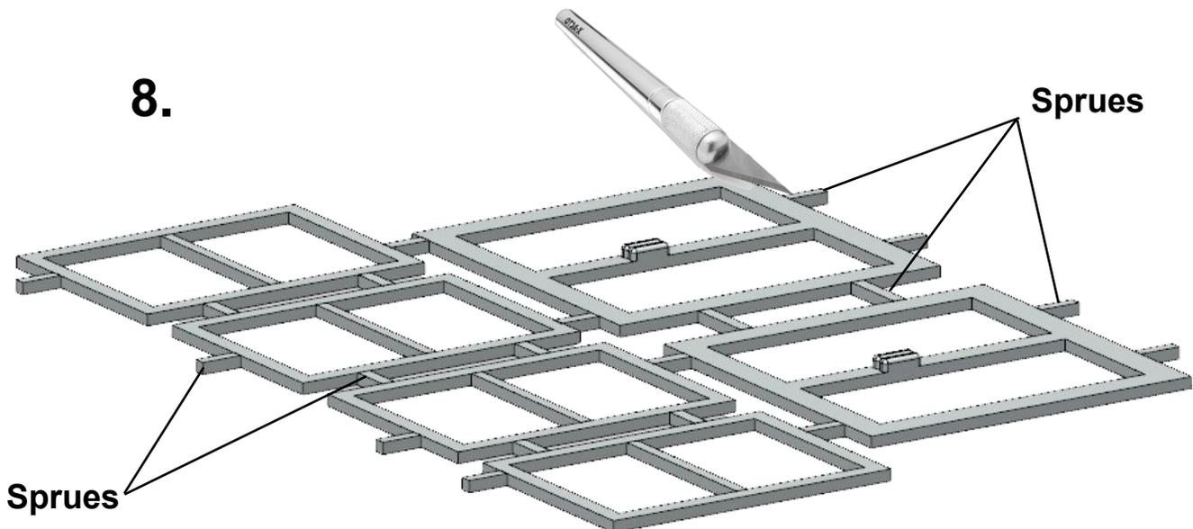
Trim away and dispose of the short attachment connectors called "sprues" from all parts. The sprues are similar to the old injection molding framework of plastic models. They make the model an integral unit which keeps the printing cost down.
