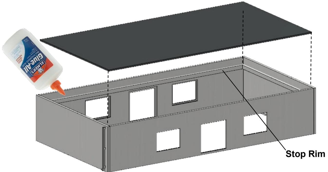
Apply a light coat of white glue along the top edge of the building's roof stop rim. Then seat the roof against the rim.
