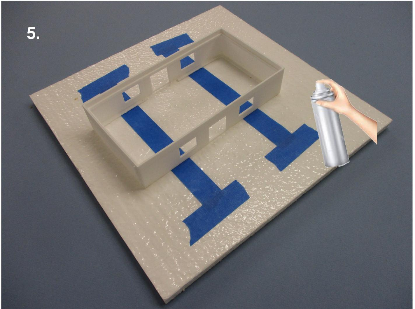
Prepare a part painting holder similar to the one shown on page-7, using styrofoam and blue painter's tape. This time, you'll only need 2-strips of painter's tape.
