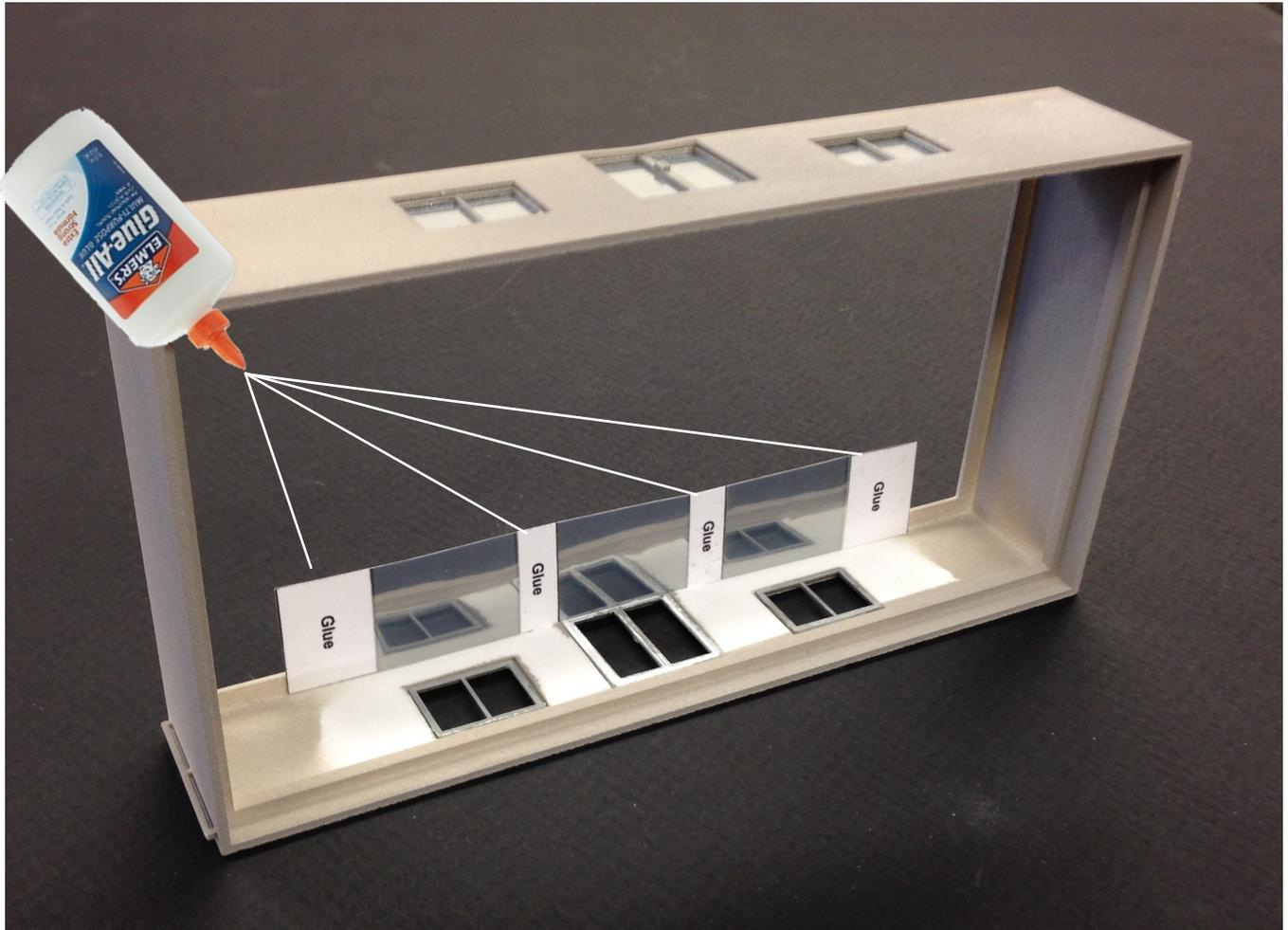
**Apply a moderate coat of glue to each area marked “Glue”, align the strip with the windows and press the strip into place.**
