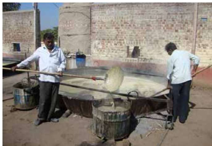
Manual removal of scum while boiling sugarcane juice in open pan
