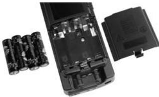
1 Place analyser on its front and open and remove battery compartment cover at the back of the analyser.
