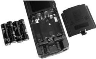
**testo 325XL:** Insert and connect rechargeable battery pack. No other steps are necessary.
