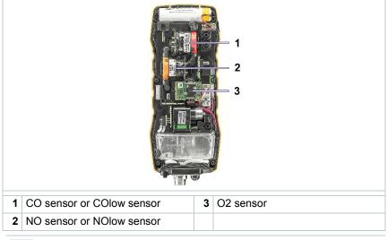
When retrofitting a sensor, the associated measurement parameter/unit must be enabled in the reading display.
