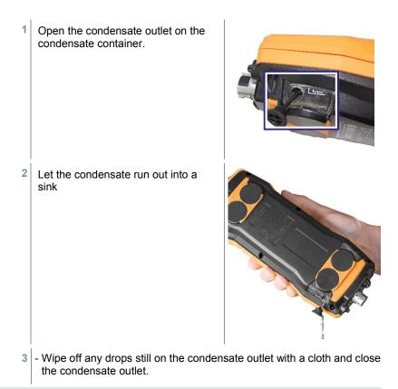
The condensate outlet must be completely closed, otherwise incorrect measurements could occur due to infiltration of external air.
