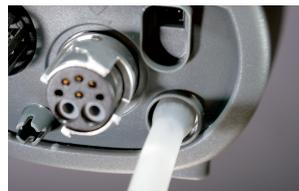
Additional differential pressure measurement up to 200 mbar
