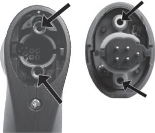
**!** Detach the flue gas probe from the measuring instrument before cleaning.
