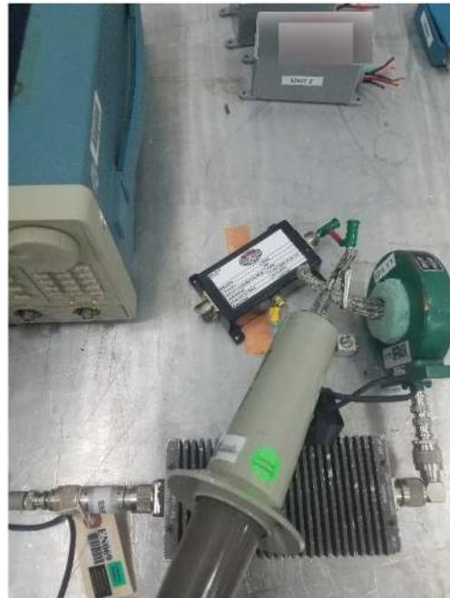
**Pulsed Current Injection****Test Setup****Short Pulse****Coax 2**
