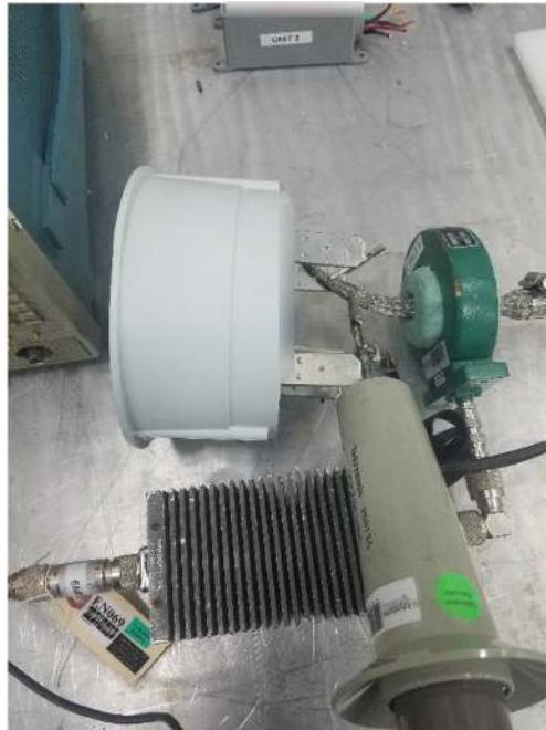
**Pulsed Current Injection****Test Setup****Short Pulse****Unit 3**
