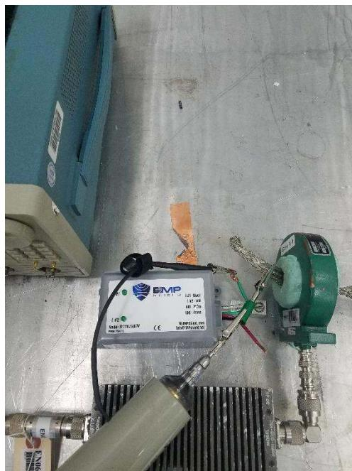
**Pulsed Current Injection****Test Setup****Short Pulse****Unit 1**
