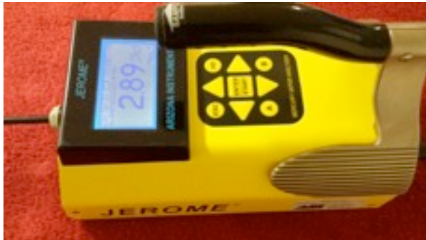
Photo 1. Unstimulated Test Results 2.89 mcg/m 3 with Jerome J405.
