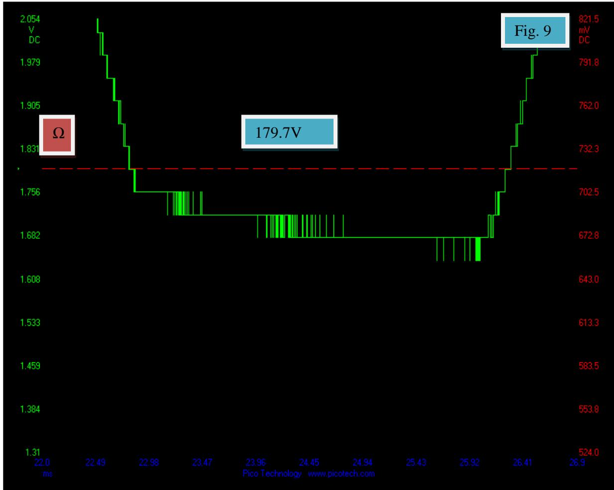
Here we zoomed in on the lower section of the curve. I am using software that has a marking accuracy of one tenth of a volt. The marker indicates, when placed precisely on the first step before the major transition: a value of 179.7 volts! Notice how the first step marks the beginning and end of a transition of major change. Also notice that the last step of the descending voltage curve equals the third step of the ascending curve.
