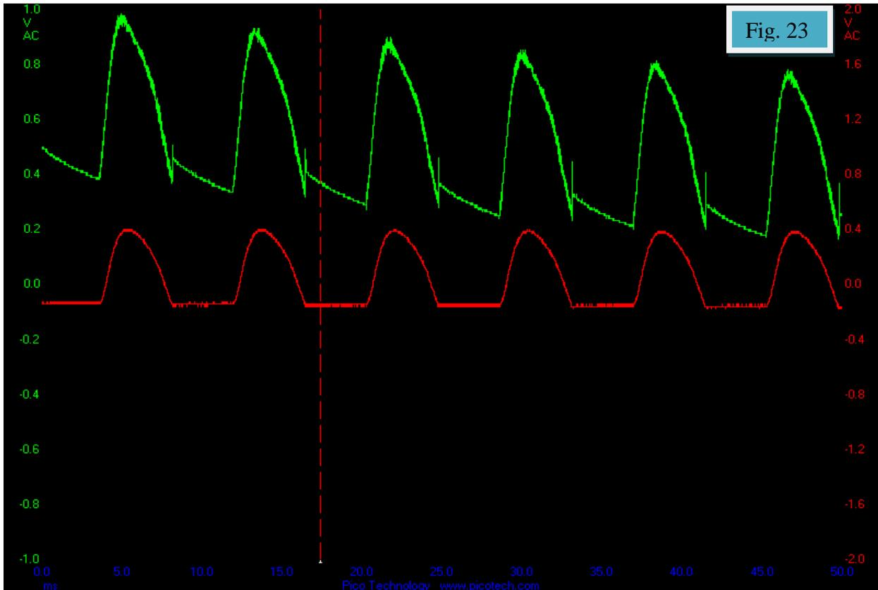
(Fig. 23) Here is another dissension pattern that occurs during a start up. The “whole curve” patterns take twice as long as the each side of the cell does to reach its “home” or steady state in the circuit.
