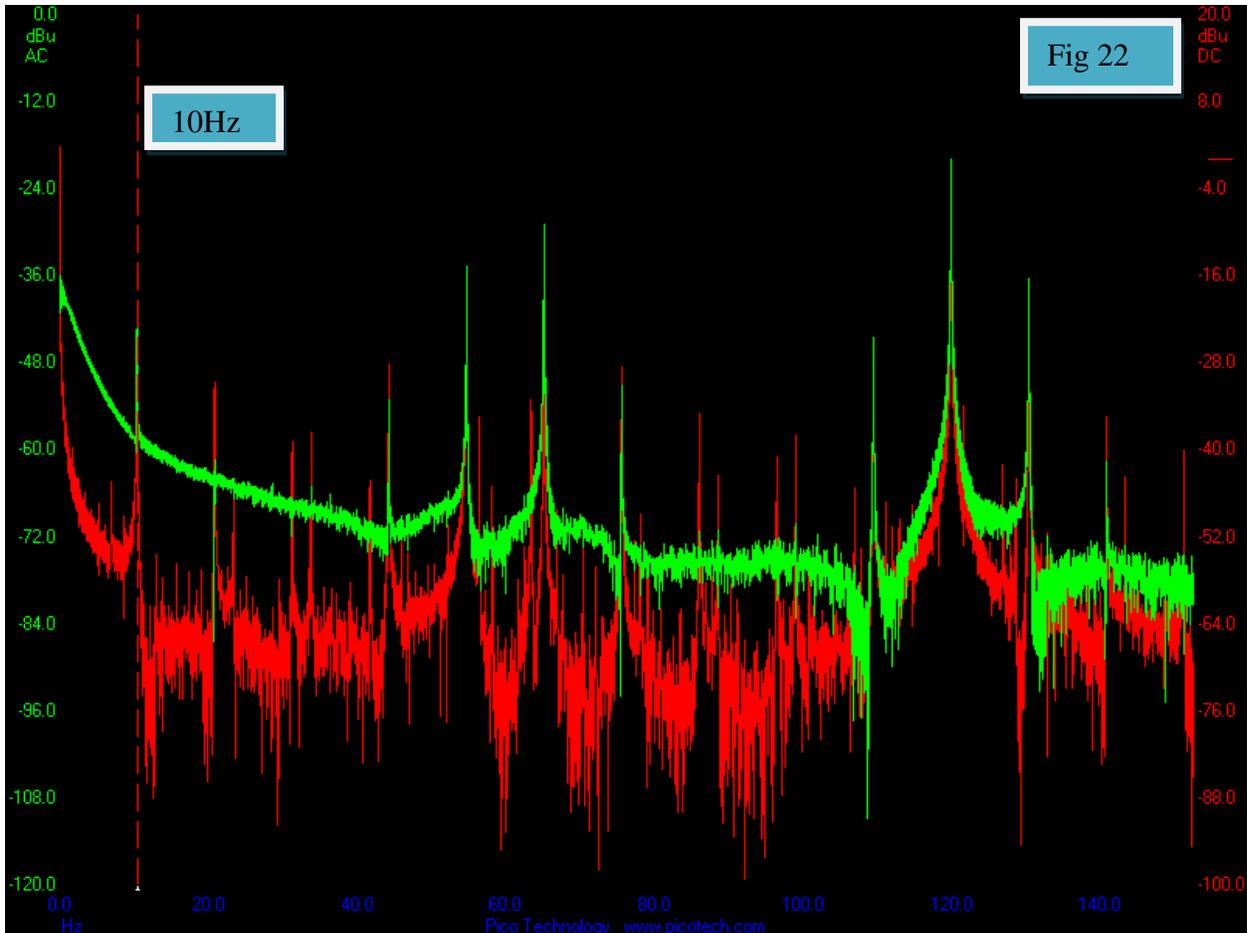
The normal noise level for the circuit is around the -48 dBu range. The mean taken over a wide band spectral reading is significantly lower when the cell is in the circuit. The marker is on the 10Hz in which there is a “near simultaneous polarity in sound”. The current responds with an abrupt change in red. The standard reference spectral curve without the cell attached is rather boring, and has a “higher” mean dBu value, by + 20, on the average.
