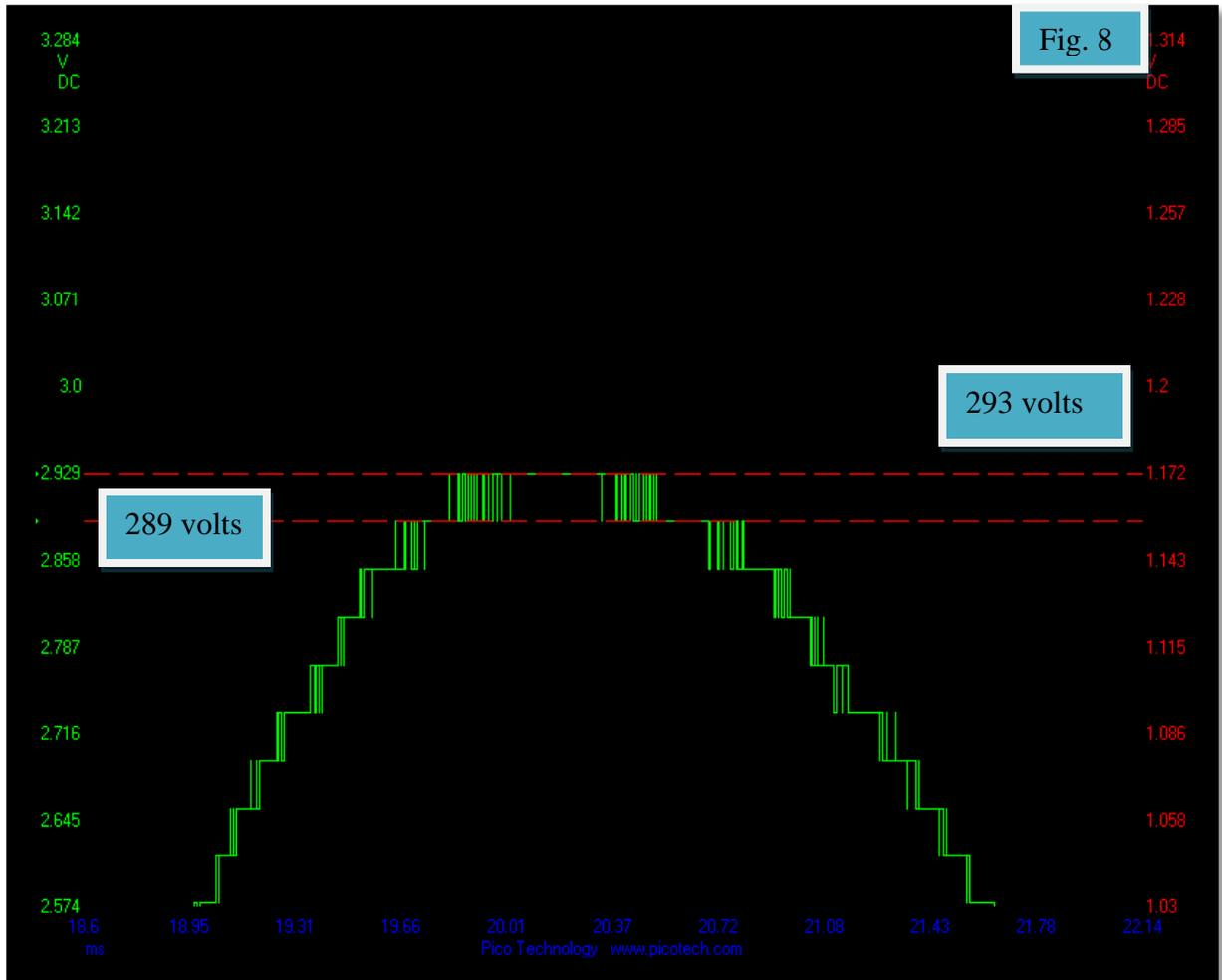
Here we have zoomed in on the peak of the voltage curve that we have been working with. The total change of the voltage is 3.97 volts in the peak area oscillations.
