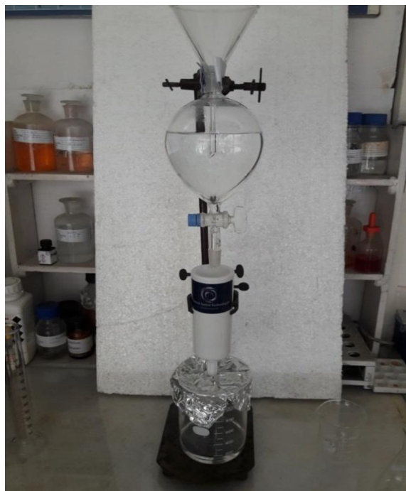
Figure 1: Structure water preparation from given device (Flow rate 12 drops/min)
