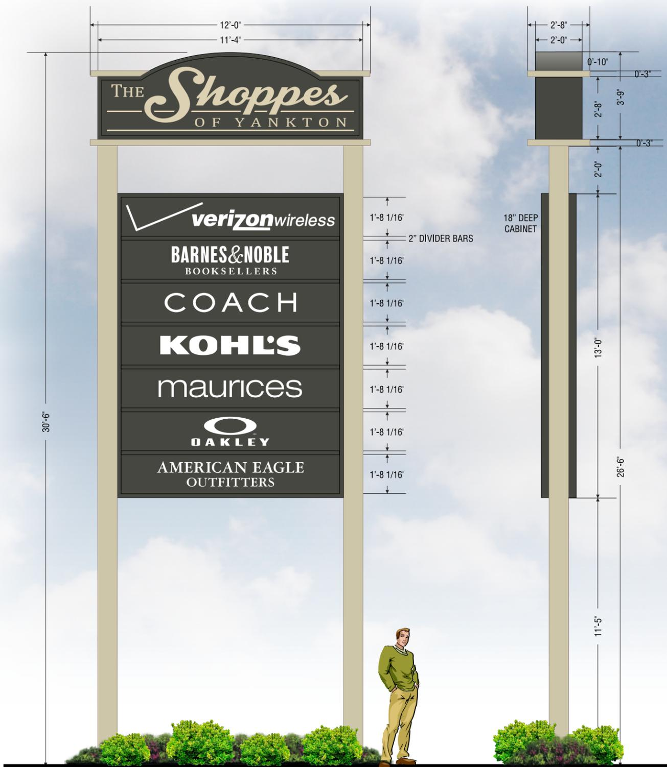
**INTERNALLY ILLUMINATED DOUBLE POLE PYLON SIGN**
