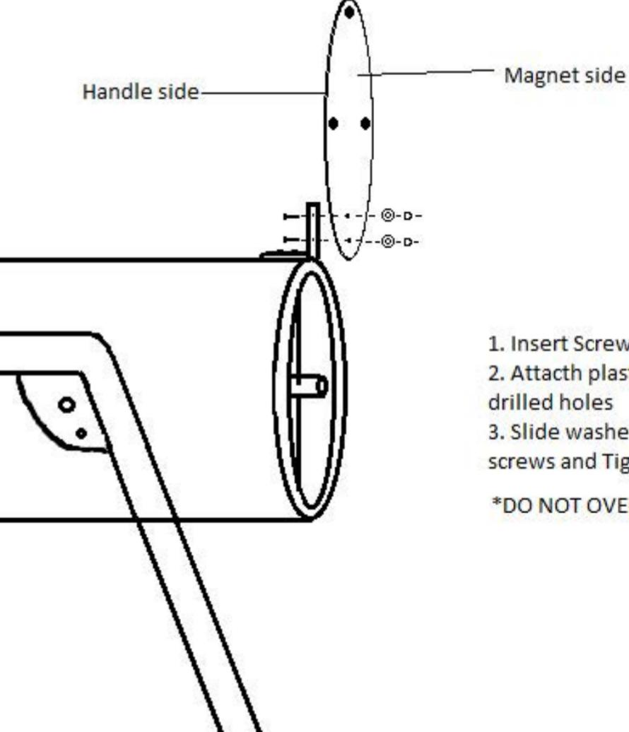
1. Insert Screws through Hinge
