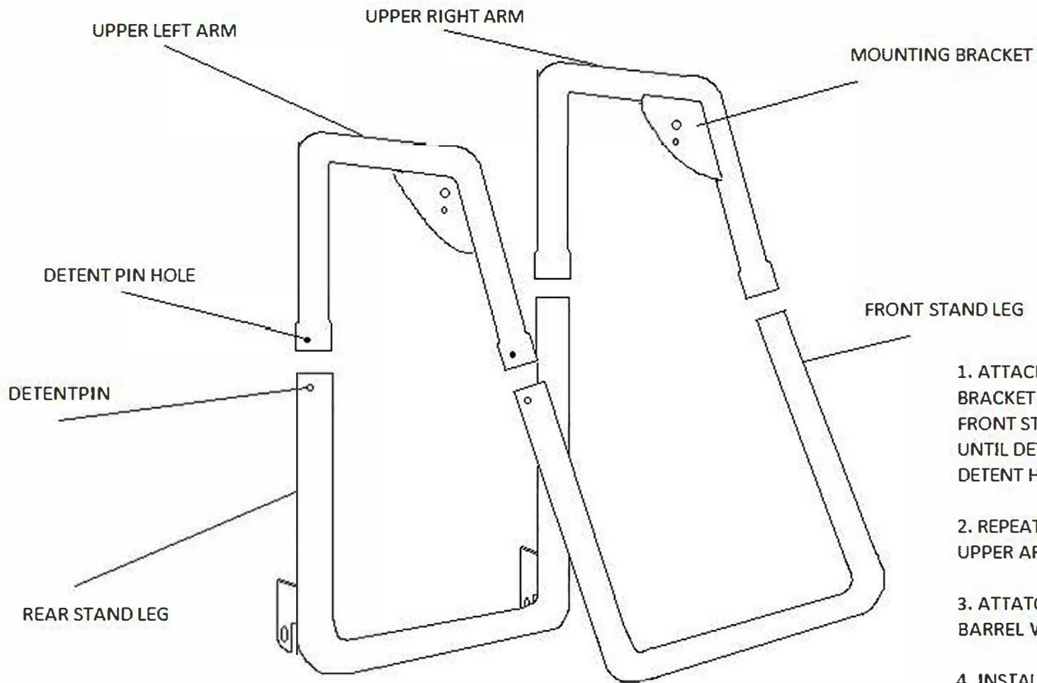
1. ATTACH UPPER LEFT ARM WITH BRACKET FACING INWARD TO REAR AND FRONT STAND LEGS AT THE SAME TIME UNTIL DETENT PINS POP THROUGH THE DETENT HOLE.
