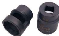
10110 12 Faces key for dismantling the electromagnet. Distance between faces 27.5 mm
