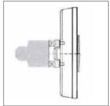
3 - Mount joint \varnothing 40 (9809-H) or \varnothing 35 (9809-HC)
