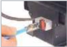
Connect compressed air (6-10 bar)
