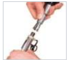
Rotate anticlockwise and release the tool ring
